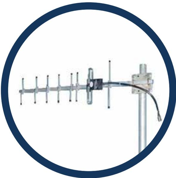
In more remote locations that may only have one cell tower which is at a distance, it is best to use a Yagi or directional antenna. A yagi antenna focuses most of its energy in the direction it is pointing. If using a Yagi antenna, you will need to know the location of the nearest cell tower. Check with your service provider.
